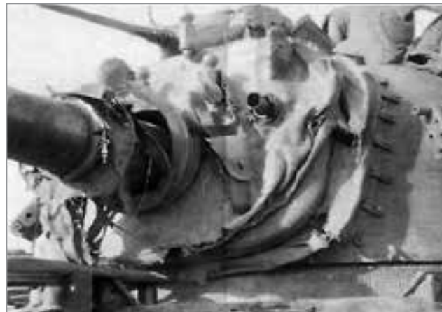
This is a photo of A-51 after a battle with the NVA where four RPGs hit her. The first RPG hit the front slope plate where the detonation blasted up towards the driver's periscope and up into the 90mm gun shield. The driver's periscope blew down into the driver face, legs and chest.
